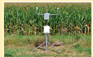
IFC's modern day hydrologic station measures rainfall, soil moisture and temperature, windspeed and direction, and groundwater levels to help improve flood monitoring and forecasting.
