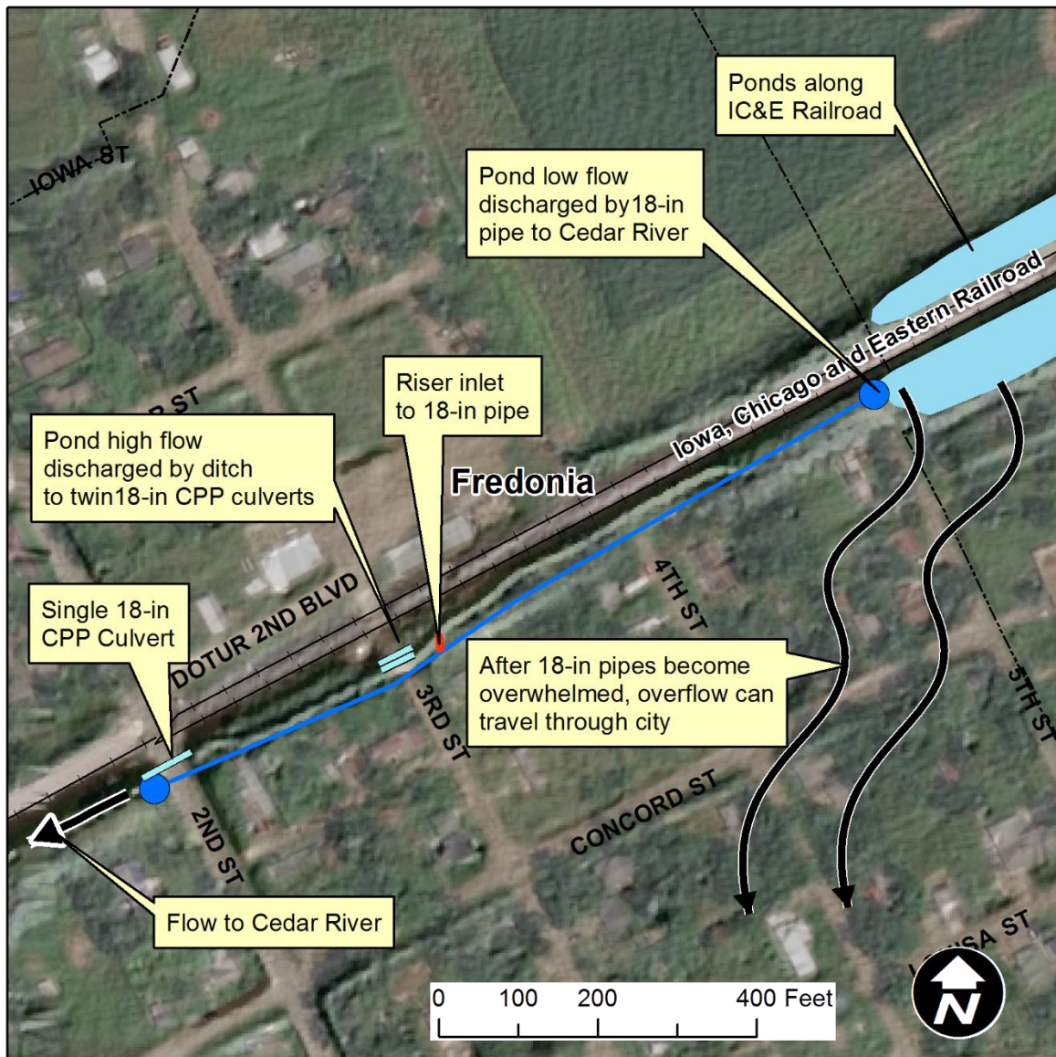
Figure 2.8. Pipes and culverts that convey pond discharge to Cedar River. Locations are approximate.
