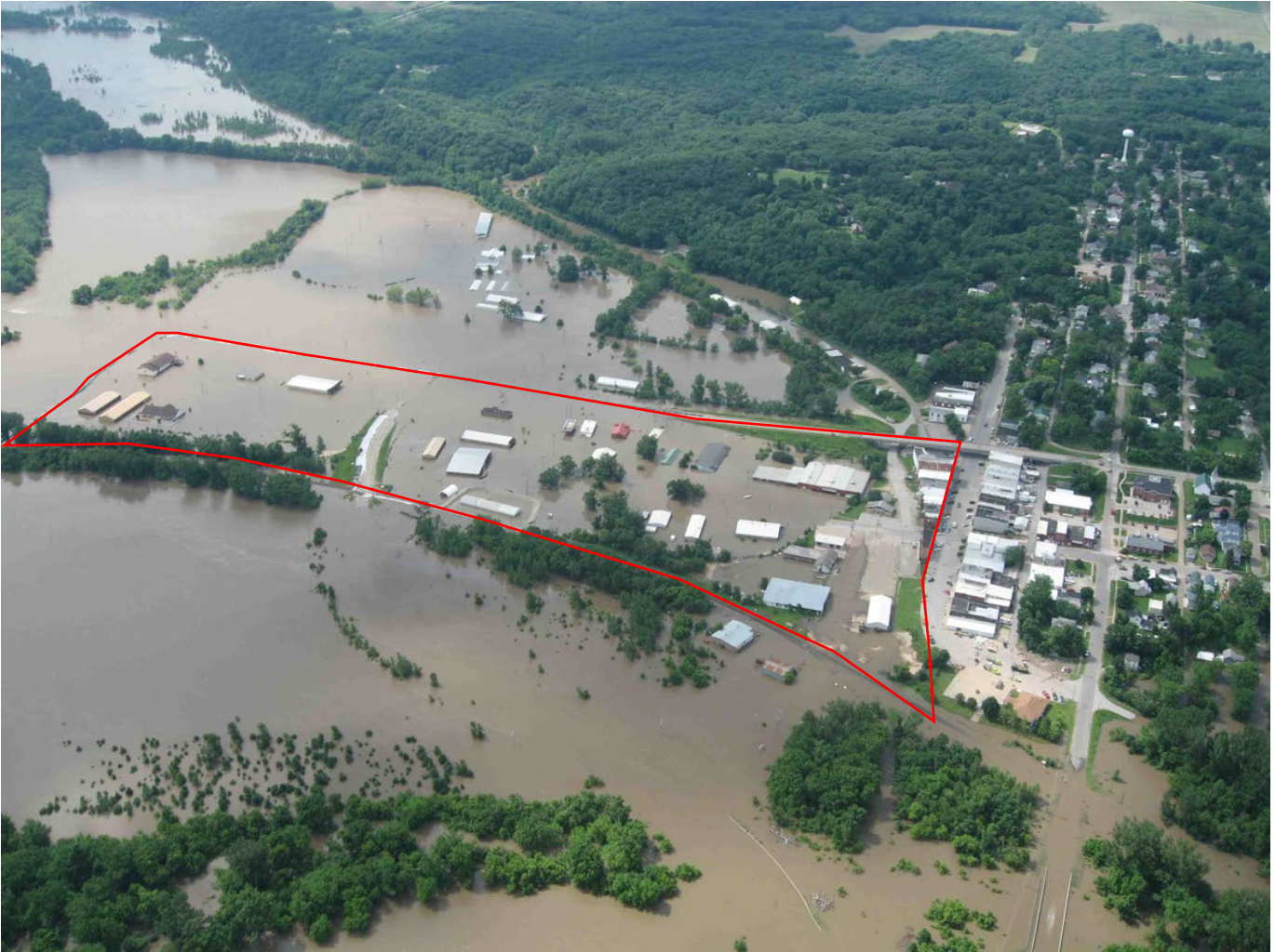
Figure 2. Columbus Junction during the 2008 Flood. The outlined area was protected by a temporary levee before its failure. Photo Credit: https://www.kenpurdy.com/FloodWeb/Flood.html
