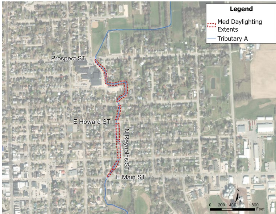
Figure 5-1. Medium daylighting project extents – uncovering buried sections, along with channel and culvert upgrades from Prospect to East Main Streets.
