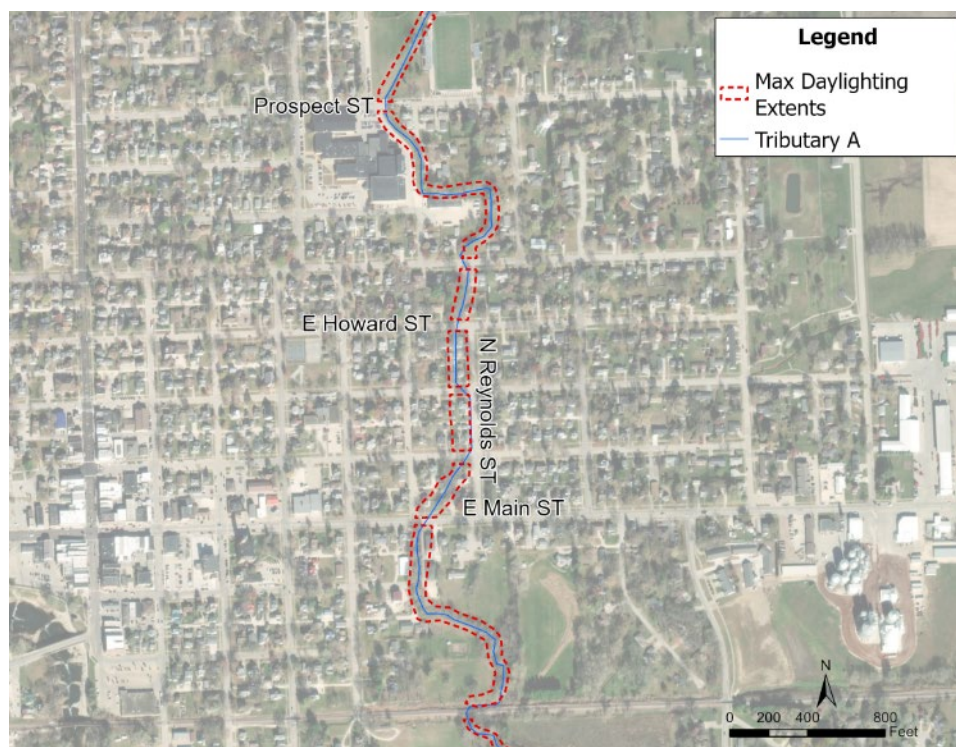
Figure 6-1. Maximum daylighting project extents – uncovering buried sections, along with significant channel upgrades and bridge replacements beginning upstream of Prospect Street to CN Railway.
