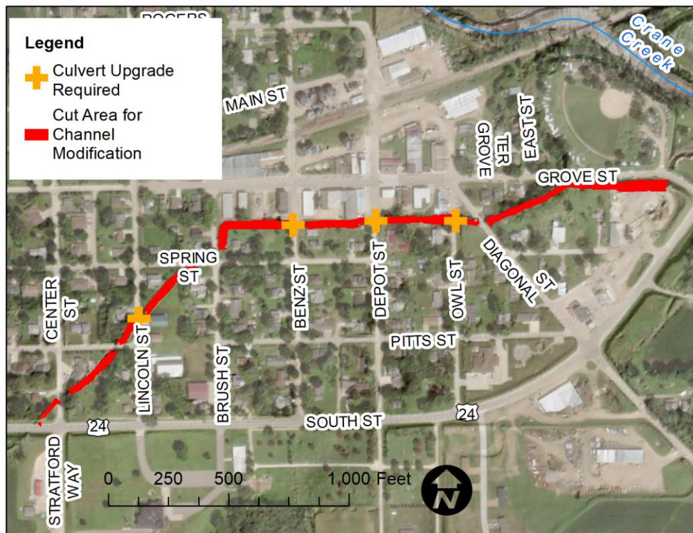
Figure 12. Cut areas required for creating a 10-foot bottom width natural channel with 2:1 (H:V) sides. Four potential culvert upgrade locations are also shown.
