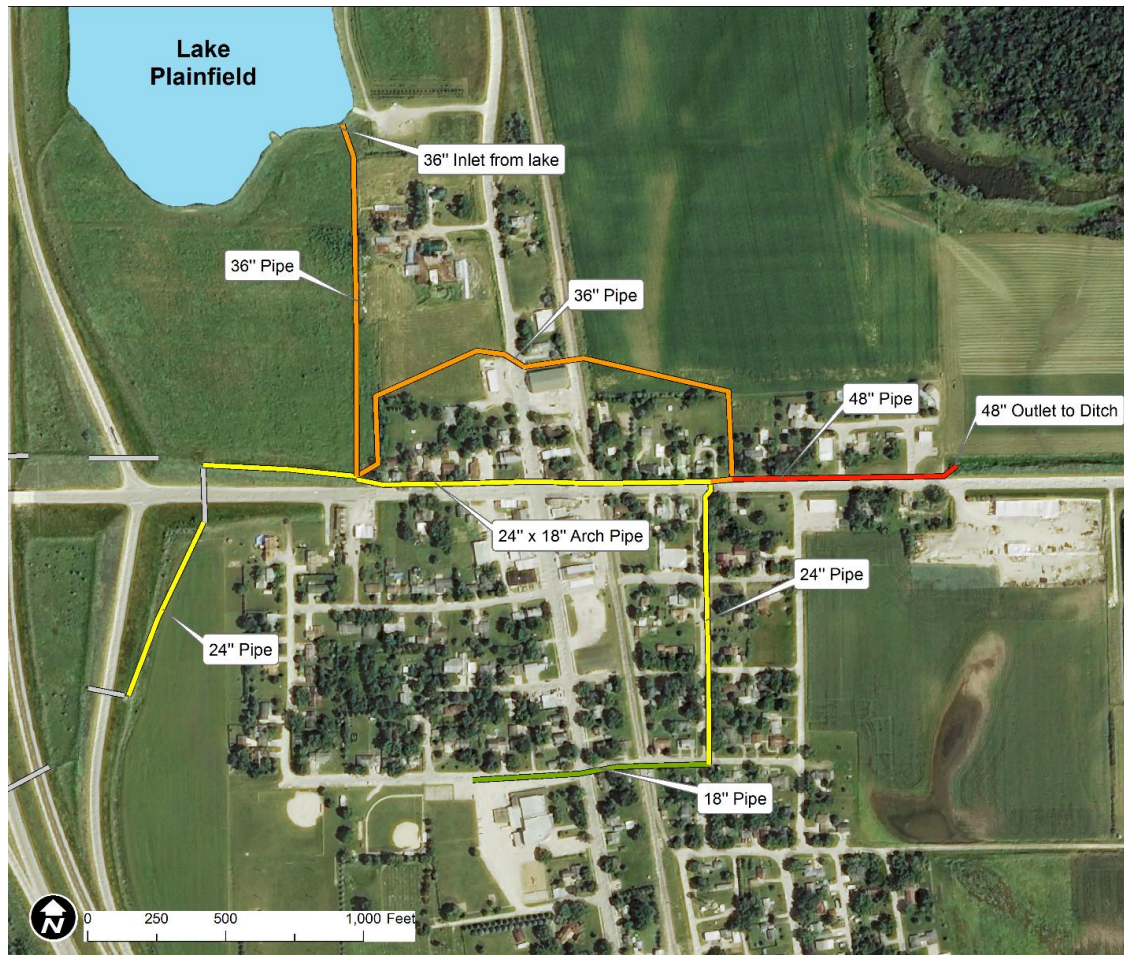
Figure 2.8. Storm sewer mains, colored by pipe size.
