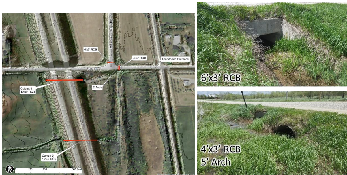
Figure 2.10. The other outlet is through culverts near the intersection of Main and 150th Streets, prior to entering the Iowa DOT wetland Mitigation Area. Photographs provided by Andy Luck.
