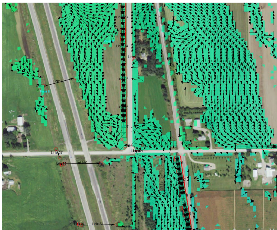
Figure 5.1. The XPSWMM model is capable of simulating rainfall-runoff, infiltration and flood through drainage system using a combination of 1D structure elements connected to a 2D grid of the terrain.
